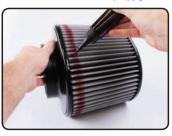
As you go, keep an eye on the amount of oil you are using and the total amount allocated for the filter. By the time you are half-way done with the
